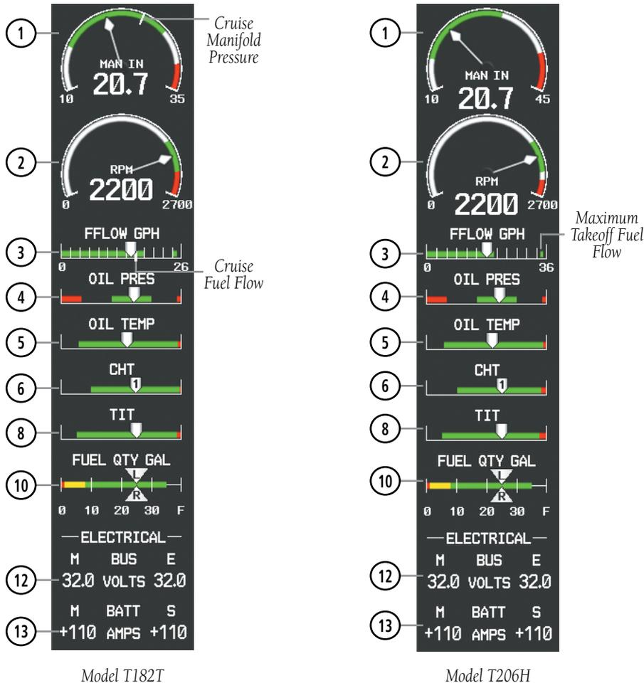
**Figure 3-2 Engine Display (Turbocharged Aircraft)**
