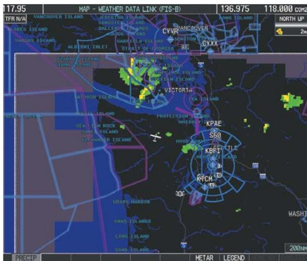
Figure 10-14 Weather Data Link Page(FIS-B) PRECIP
