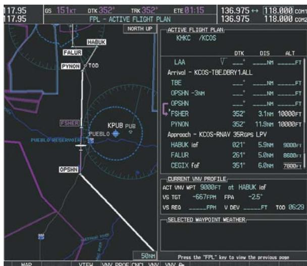
Figure 7-42 Tracking the OPSHN to FSHER Leg
