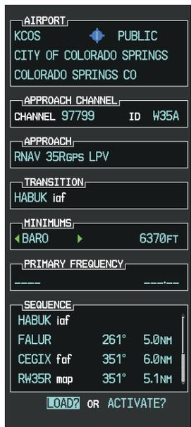
Figure 7-33 Barometric Minimums Set
