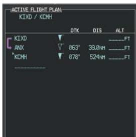
Figure 8-17 Airway Entry Point Loaded
