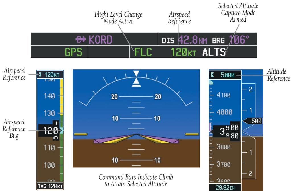
**Figure 6-9 Flight Level Change Mode**
