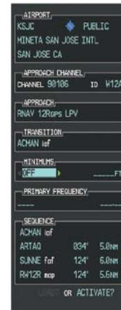
Figure 9-8 Selecting Barometric Altitude Minimums
