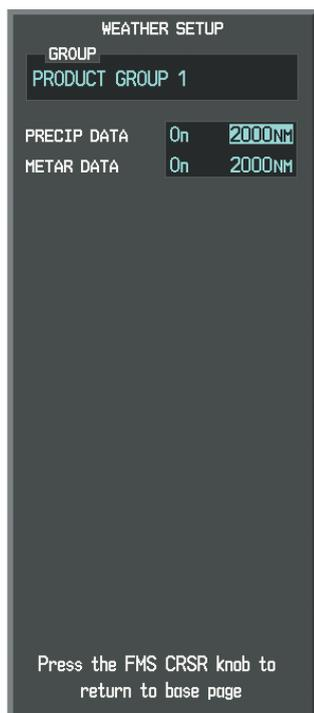
Figure 10-10 Weather Data Link Page Setup Menu
