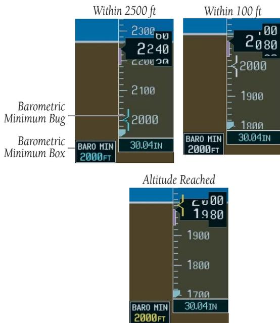
Figure 2-17 Barometric Minimum Descent Altitude Alerting Visual Annunciations
