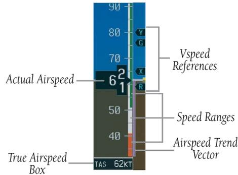
Figure 2-4 Airspeed Indicator
