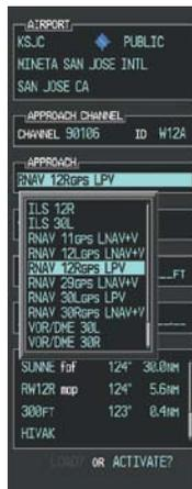
Figure 9-6 Selecting an Approach Procedure
