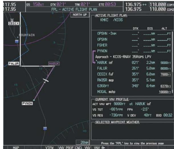
Figure 7-46 Descending Turn to the Initial Approach Fix (IAF)
