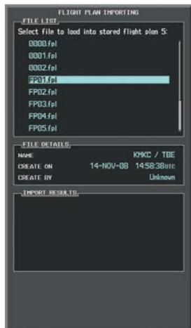
Figure 8-13 List of Flight Plans to Import
