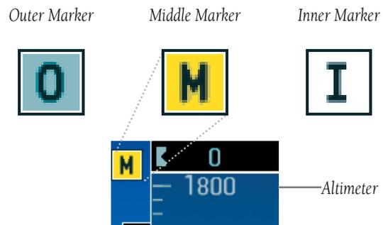
Figure 5-4 Marker Beacon Annunciators on the PFD
