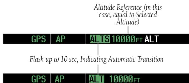
**Figure 6-6 Automatic Mode Transitions During Altitude Capture**
