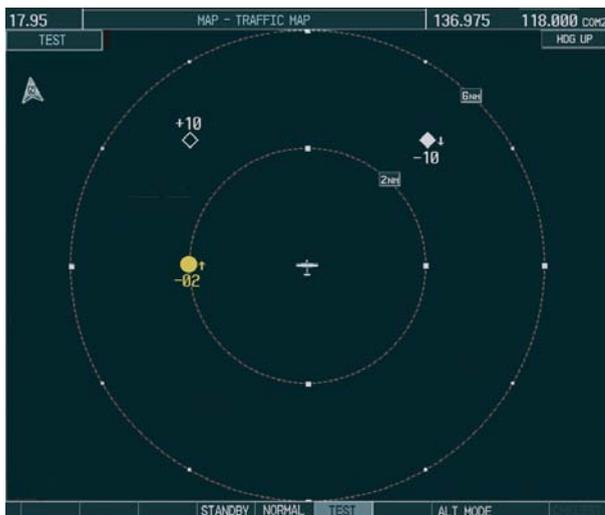
Figure 10-33 Self Test OK Display
