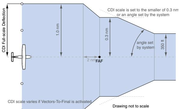
Figure 2-23 Typical LNAV and LNAV+V Approach CDI Scaling
