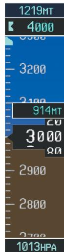
Figure 2-9 Altimeter (Metric)
