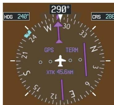
Figure 7-12 Assigned Heading of 290°
