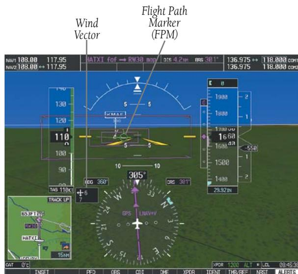
Figure 11-6 Flight Path Marker and Pathways
