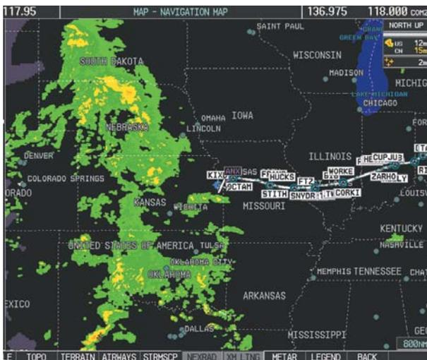
Figure 10-6 Navigation Map Page Displaying NEXRAD Weather
