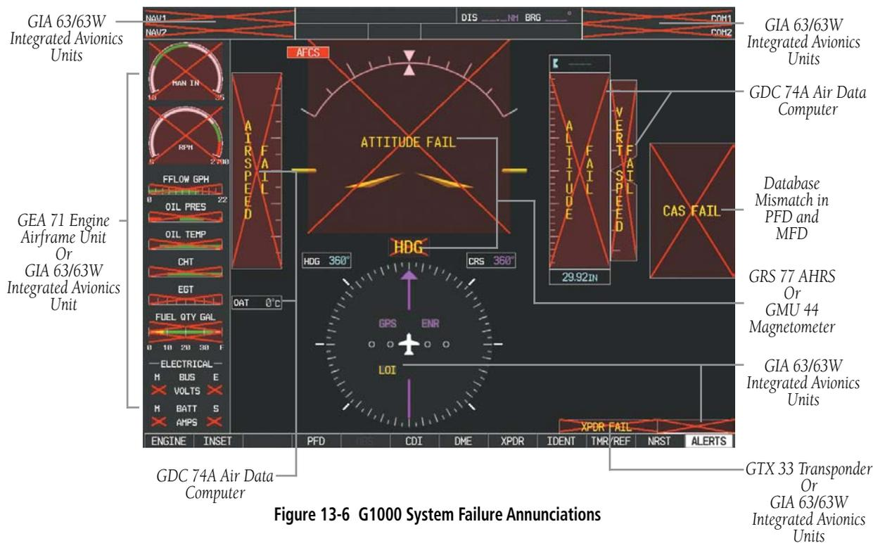
**Figure 13-6 G1000 System Failure Annunciations**
