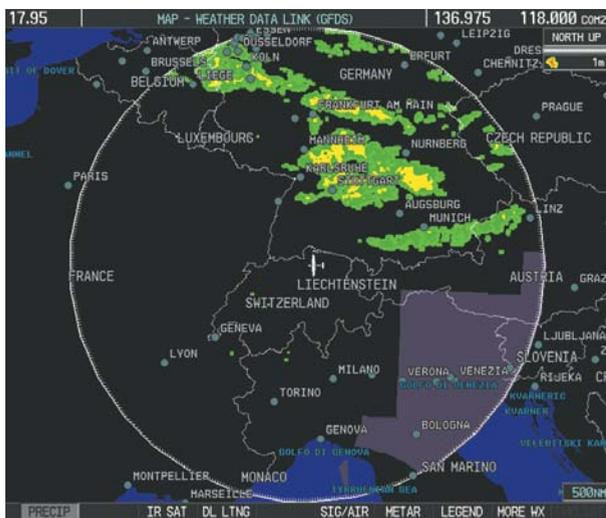
Figure 10-28 Weather Data Link Page (GFDS) PRECIP
