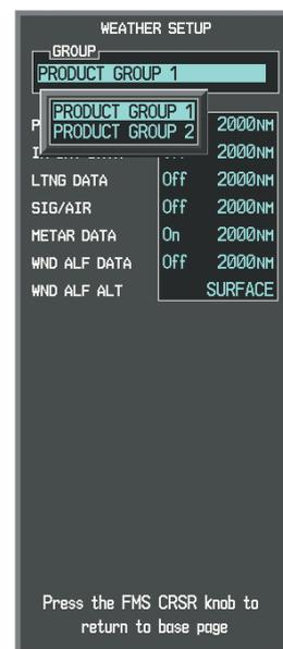
Figure 10-18 Weather Data Link (GFDS) Page Setup Menu
