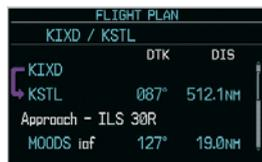
Figure 8-2 Active Flight Plan Window on the PFD
