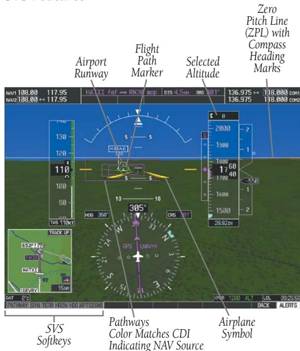
Figure 11-2 SVS on the Primary Flight Display
